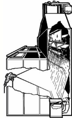
Figure 2 - Waterwash Industrial Type Spray Booth
